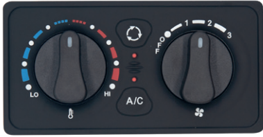
Manual Control Unit - 3 Blower Speeds - A/C and Recirculation Push Buttons
